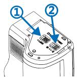
To remove SD card from the camera, unlock the security lid by sliding the latch on the compartment lid (1) and then open the lid by pulling the second latch (2).
